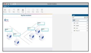
The graphical, web-based editor lets you intuitively implement plant layouts, integrate customized reports, or display measured values, operating states, or produced quantities in real time, for example. Any end device with an appropriate internet browser can be used for display, be it a tablet or a large ANDON tablet.
