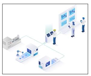
Modern production facilities usually have an Ethernet port that allows them to be connected to a Local Area Network (LAN), which can then be used to read out the relevant machine data using fieldbus protocols. If this is not the case, it is usually possible to install so-called communication processors or adapters. Digital and analog signals can also be recorded directly via fieldbus controllers.
