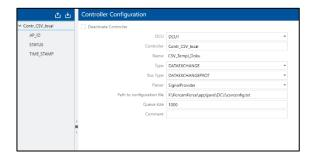
Depending on the control and fieldbus type, DCUs can operate up to 100 controllers of different types simultaneously without special requirements on the PC hardware on which they are installed. To increase the availability of such a system, two DCUs can be configured simultaneously to monitor each other. If one DCU of the pair were to fail, the DCU that is still functional then automatically takes over the tasks of the failed DCU (failover). If a
