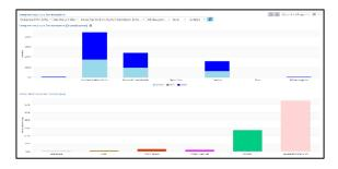
Evaluating the energy consumption per operating state provides information on how much energy and other resources were consumed during and outside of production. It indicates the exact amount of consumption for each operating state.
