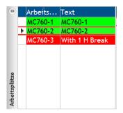
The BDE view exists in the upper half of two tables. The left table shows the workplaces assigned to the currently selected terminal. Depending on which workplace has been selected in the left table, the right table will show a list of operations that have been assigned to it.
