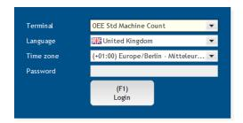
When logging into the Shop Floor Terminal, you need to enter the terminal itself, the terminal language as well as the time zone, and - if necessary - a password.
