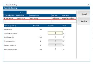
Through the Shop Floor Terminal, you can select whether automatically measured quantities should be categorized as material quantities, scrap quantities, or rework quantities along with a qualifying reason for each. The list of scrap and rework reasons can be tailored to a client's specific requirements.
