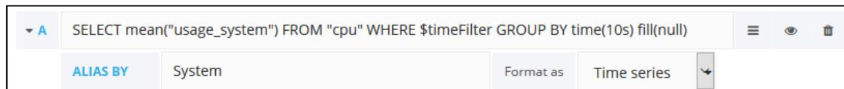
A screenshot of the Grafana query editor. The query field contains: `SELECT mean("usage_system") FROM "cpu" WHERE $timeFilter GROUP BY time(10s) fill(null)`. Below the query are buttons for **ALIAS BY** (highlighted), **System**, **Format as**, and **Time series**.
