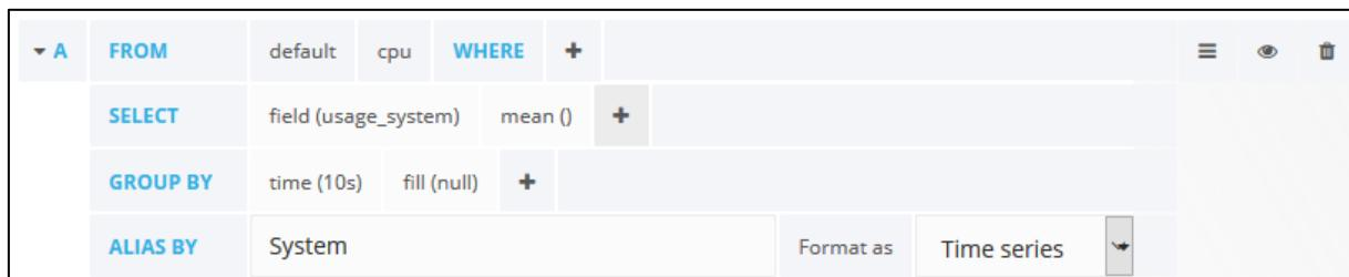
**Fig. 18: Configuration of a metric displaying the system's CPU load**
