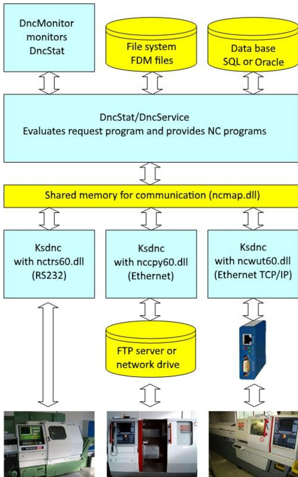
Figure 1: Transmission of NC programs to the machine with FORCAM FORCE™ and back
